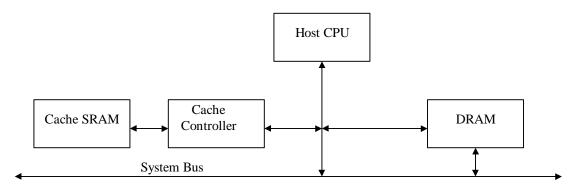
This design does not isolate the processor bus from the system and the memory bus. When the processor initiates a bus cycle, all devices in the system immediately detect the bus cycle address. The cache controller monitors each memory access request to determine if it has a copy of the requested information. If there is a hit, the controller terminates the bus cycle in zero wait states and also instructs the memory subsystem to ignore the request. To summarize:
